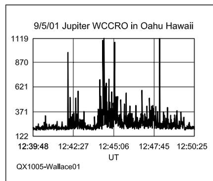
Figure 1 — Jupiter radio noise bursts received at 20.1 MHz using a Jove receiver and dual dipole antenna. Signals are displayed using SkyPipe software. The vertical axis is proportional to voltage.
